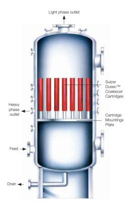
Sulzer Dusec Coalescer Mounting Plate and Cartridges
